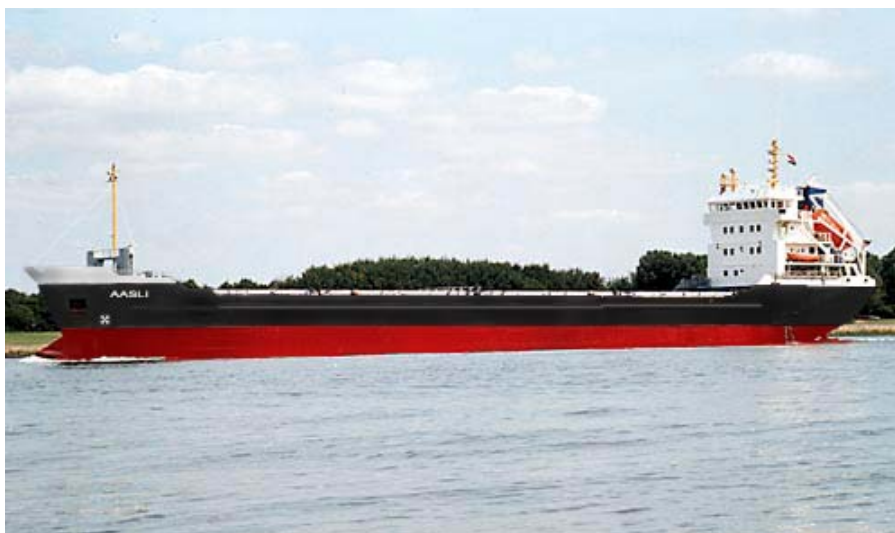
Figur 2.3 Bulkskipet Aasli, 6.630 dwt, selvlosser, Aasen Shipping AS – byggeår 1994
